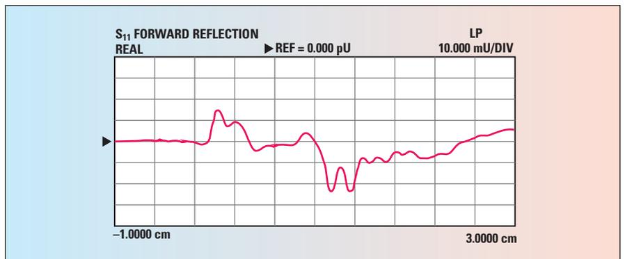
▲ Fig. 5 Gated  $S_{11}$  in TD of the 110 GHz connectors 01K80A-40ML5.
